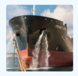
Ballast water is fresh or salt water held in the tanks and cargo holds of a ship. It is used to provide stability and mobility during a journey.
